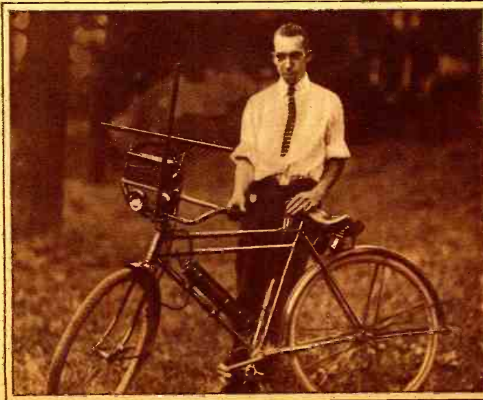
The compact portable receiver with its loop mounted on the handlebars of the bicycle has, it is claimed, a range of 100 miles. The batteries for the set are carried in the metal case on the frame of the bicycle. Photos © Herbert, Inc.
