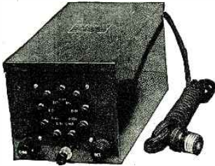
An A.C. "B and C" eliminator employing an electrolytic rectifier. The detector tap is variable from 0 to 80 volts. Other taps provide 45, 67, 90 and 135 volts. "C" voltages from 0 to 40 are obtainable.
