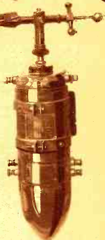
This is a close-up of the generator, a 24 propeller which drives it, to furnish current for the main transmitting set. The single blade is used for better regulation of the speed, which must not vary with that of the plane.
