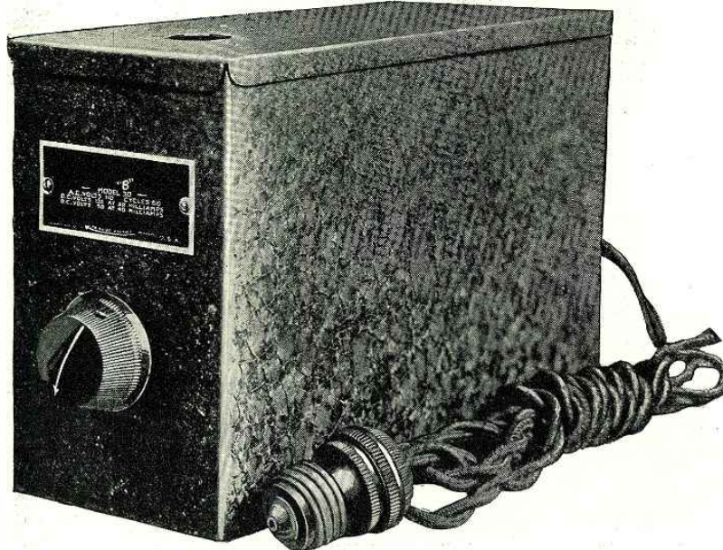
A "B" eliminator designed for use on a 110-volt 60-cycle light line. It employs a full-wave rectifier tube of the filamentless type. There are four voltage taps: detector, variable from 20 to 60 volts; radio-frequency, variable from 67½ to 90 volts; and high- and low-voltage taps, controlled by a switch, for the audio amplifiers, giving a maximum of 180 volts for a power tube.
