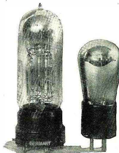
Comparative sizes of a 201-A type tube (right) and the Loewe multiple tube (left).
