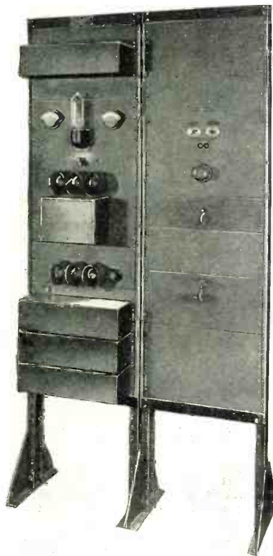
Fig. 4 A Carrier-Current Telephone panel unit, for use in connection with high-voltage power-transmission lines.
