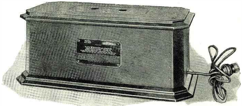
An A.C. "B" eliminator employing a full-wave rectifier tube and a voltage-regulator tube to compensate for irregularities in line voltage. There are four voltage taps; namely, 22½, 45, 90 and 135 volts. The maximum current obtainable is 50 milliamperes, sufficient for most purposes. Regardless of the load placed on the eliminator, the voltage remains constant.
