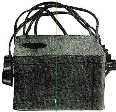
An A.C. "B" eliminator employing a half-wave rectifier tube and supplying a variable detector voltage from 0 to 75, radio-frequency voltage 0 to 90, and amplifier voltage from 0 to 135.
