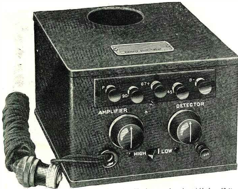
An A.C. eliminator using a full-wave rectifier tube. The detector voltage is variable from 10 to 60, the radio-frequency tap from 67 to 90. Maximum amplifier voltage is 135. A high-and-low voltage switch is also incorporated; the high-voltage side is used when 6 or more tubes are employed in the receiver.
