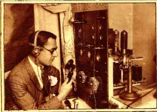
Above is a close-up of 2-ABT's 300-watt transmitter. Notice the fine workmanship in both the transmitter and receiving apparatus, in this and the illustration at the right. It is said that this station cost in the neighborhood of five thousand dollars. © Herbert Photo.
