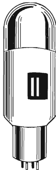
A rectifier tube filled with gas will flash on the application of suitable voltage and may be used in television experiments.
