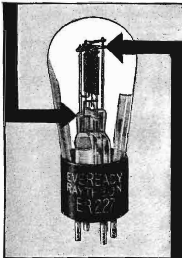
Showing the exclusive, patented Eveready Raytheon 4-Pillar construction. Note the sturdy four-cornered glass stem, the four heavy wire supports, and the bracing by a stiff mica sheet at the top.
