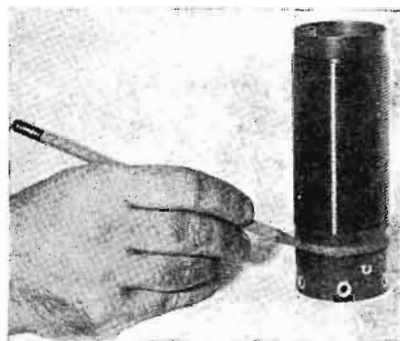
Fixed coupling between secondary and tickler coils makes it possible to calibrate detector tuning circuits with a fair degree of permanency and accuracy
