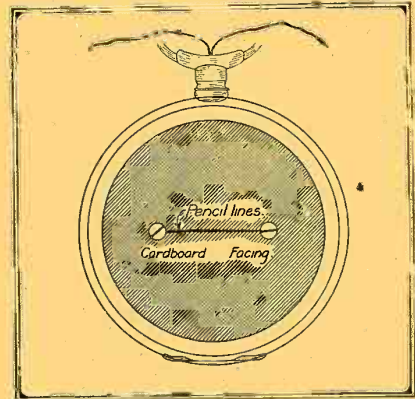
Every Real Boy Has an Old Dollar Watch Laying Around. Use the Case For a Grid Leak.
