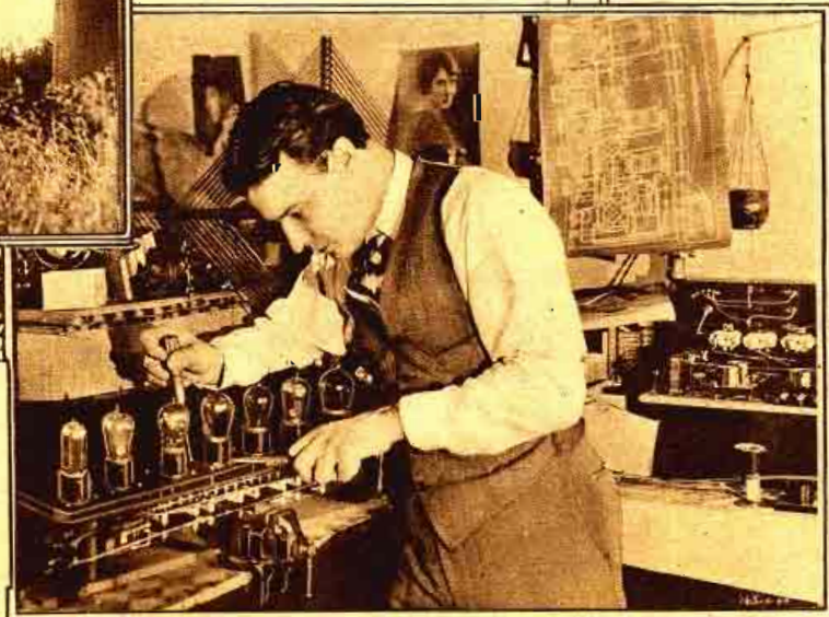
Robert Fraser, well known movie star, is an enthusiastic radio fan. He has equipped a corner of his garage with the necessary tools and has built a great many sets in this workshop. He is seen here putting the last touch to a Super-Heterodyne.
