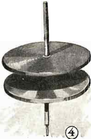
A "capacity" is formed by the proximity of any two conductive surfaces just so long as there is a non-conductive space between them. Such an arrangement is called a condenser.
