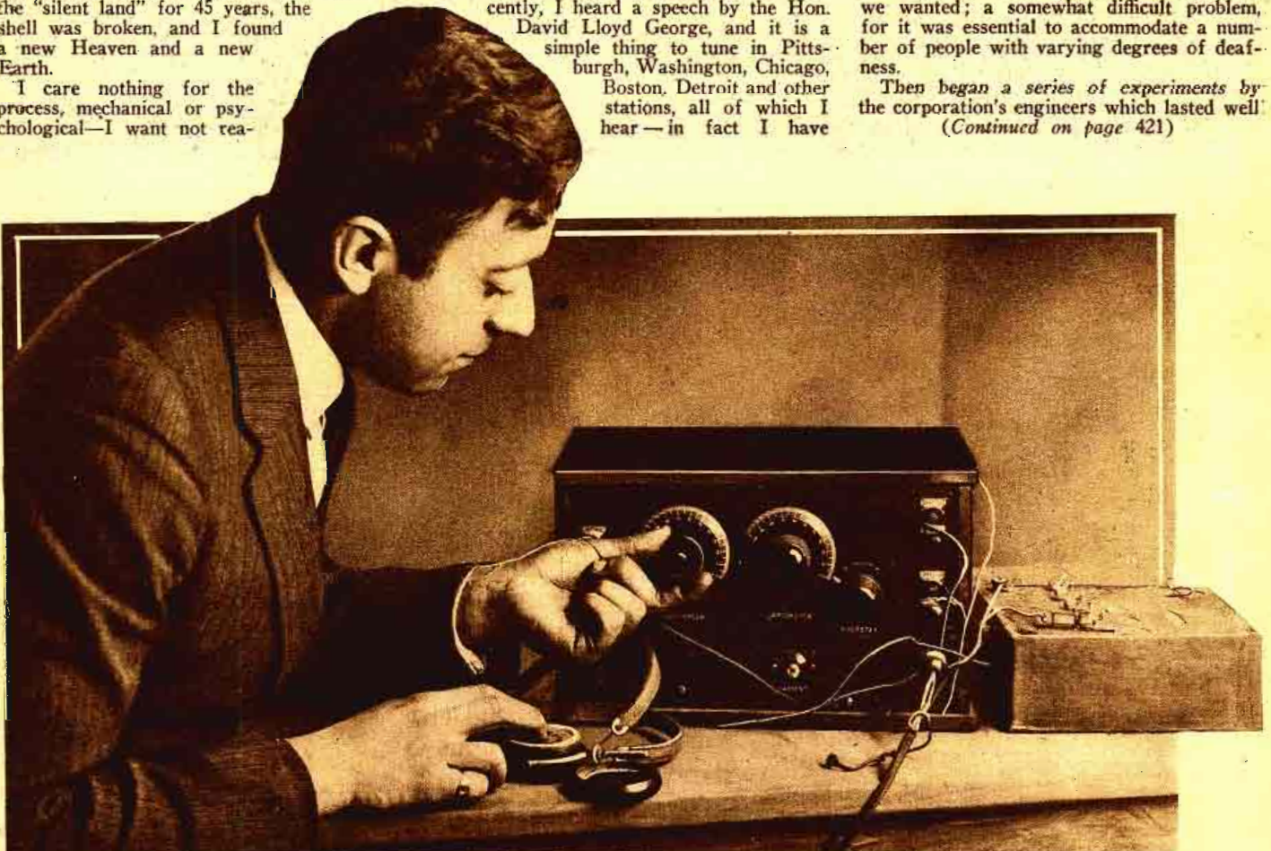
We should like to cite the case of Mr. H. Dufony, of Jersey City, who, though deaf, finds it possible to hear everything that comes over his radio set by unscrewing one of the caps of his phones and lightly touching the diaphragm with his fingers. ©Photonevs, N. Y.
