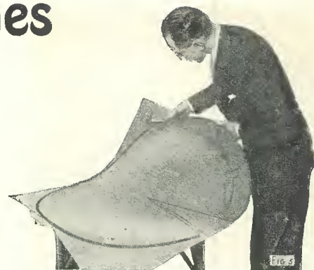
Fig. 5 illustrates the paper diaphragm being cut out, preparatory to gluing and mounting.
