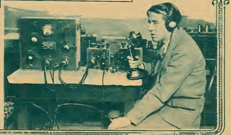
At the left, Prof. H. H. Henline of the department of electrical engineering, Stanford University, California, standing beside equipment of the university's experimental radio station 6XBM. This station has two transmitting sets, long- and short-wave, with which it has sent out standard-frequency signals, aiding in the work of the Bureau of Standards. One ranges from 50 to 200 meters, and the other from 200 to 2,400. © UNDERWOOD & UNDERWOOD.
