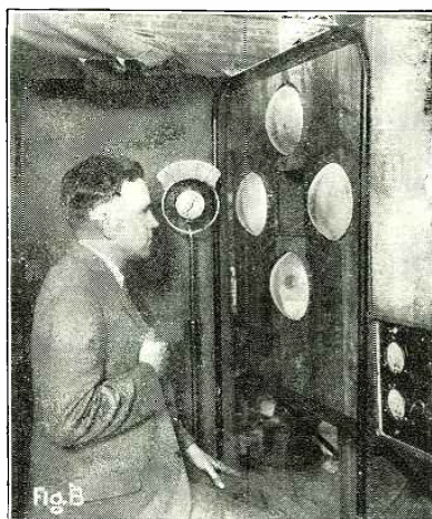
M. L. Hayes, seated before the photoelectric cells of WCFL's television transmitter.
