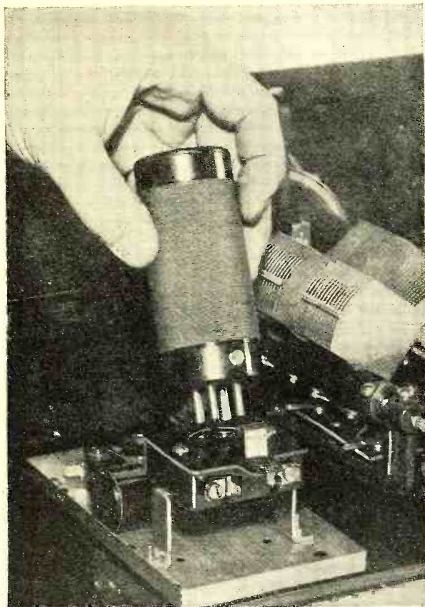
THIS DETAILED VIEW OF THE DETECTOR SHIELD CAN SHOWS THE TERMINAL PLATE WHICH FITS OVER THE COIL SOCKET TO ACCOMMODATE THE DETECTOR COIL WITH ITS TICKLER WINDING
