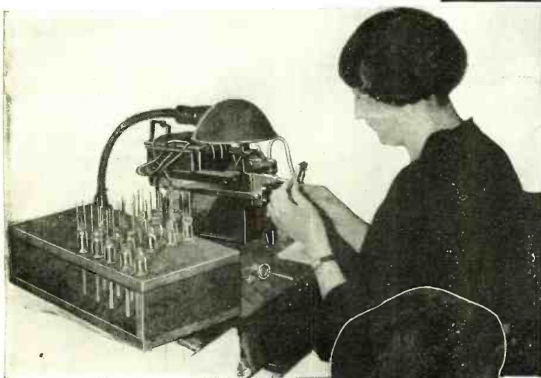
¶ Fig. 5—By Means of gauges, the operators assemble the grid, plate and filament elements for spot-welding to the sealed-in lead wires
