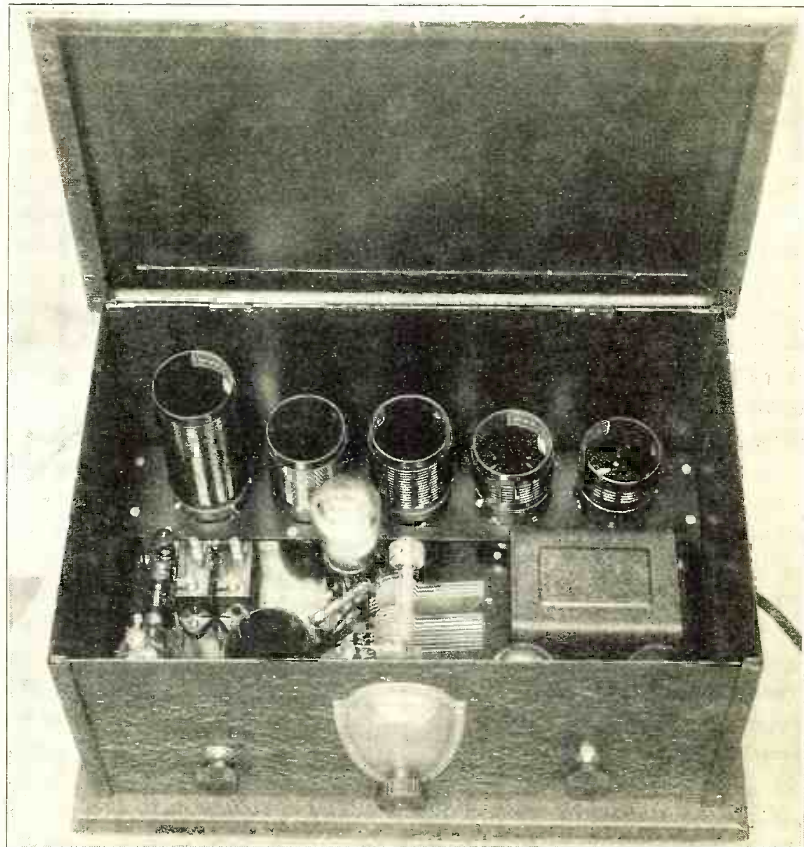
AN INTERIOR VIEW OF THE NATIONAL SHORT-WAVE RECEIVER, WITH THE REMOVABLE COILS FOR DIFFERENT WAVE BANDS READILY ACCESSIBLE
