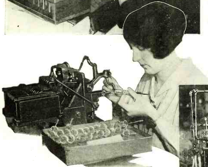
¶ Fig. 6—Here the assembled elements are being welded into place; accuracy of spacing between the elements being assured by the gauges shown in Fig. 5
