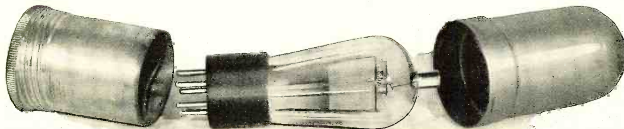
BELOW—THIS SHOWS HOW THE A.C. SCREEN-GRID '24 TUBE IS INSERTED IN THE TUBE BALLAST SHIELD
