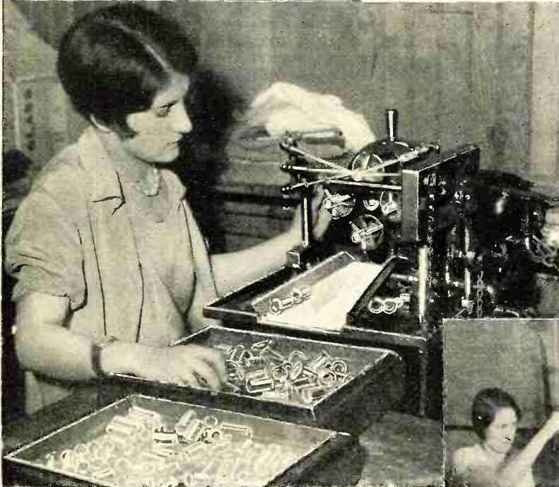
¶ Fig. 2—A Machine for flaring the glass tube which acts as a support for the tube elements. This machine, ingenious and costly as it is, is already being superseded by one incorporating even greater cost-cutting improvements
