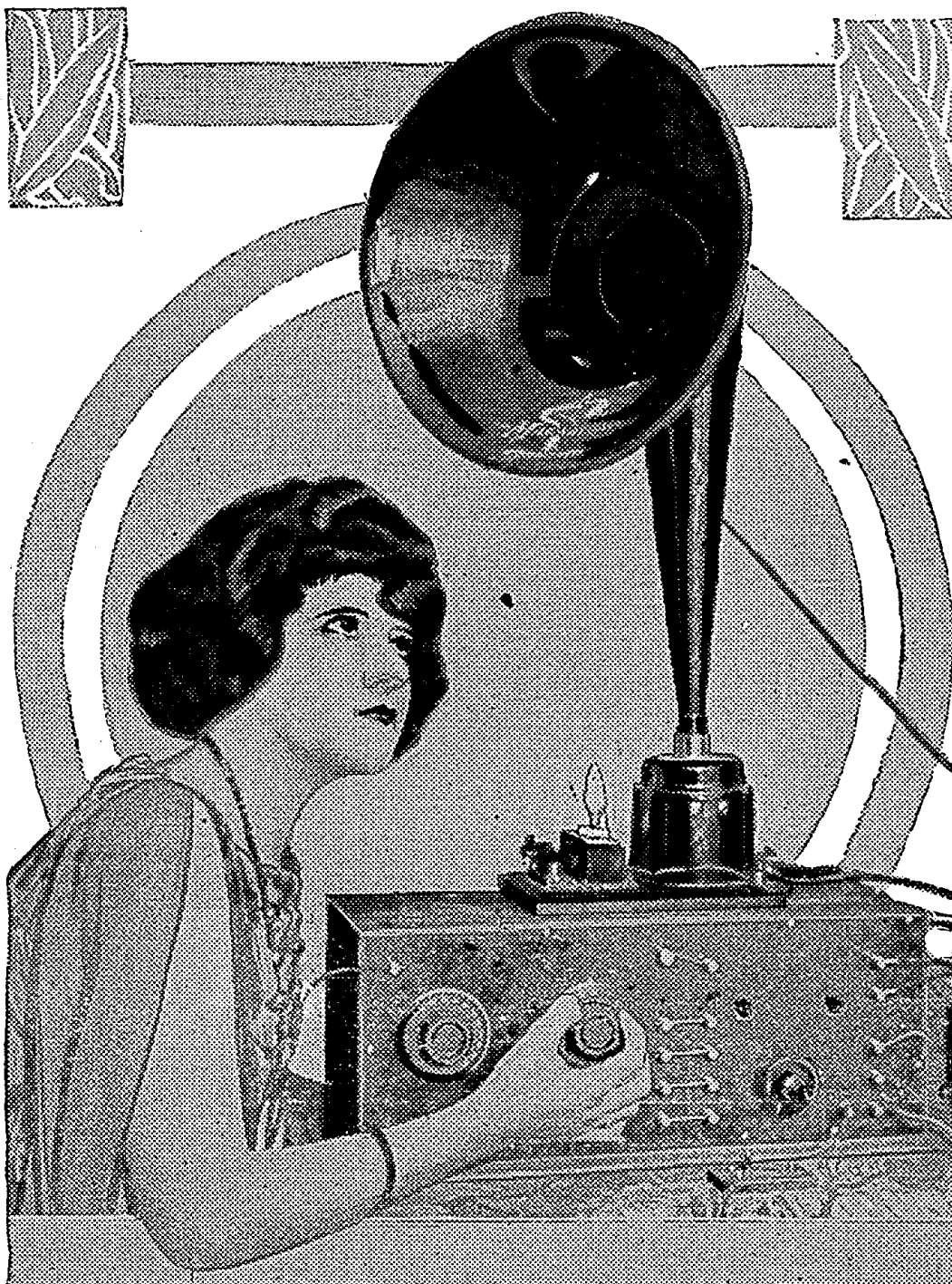
The Radiophan rushing to bed after a late concert is apt to forget to disconnect the battery wires of the power speaker. This is especially possible where (as in many cases) a separate battery is used for coil excitation. To prevent this, this pretty Radio Miss has placed a small six-volt lamp in parallel with the power speaker, and the burning of same is a continual reminder that the current is on. Result: no rundown batteries next morning © K. E. H.
