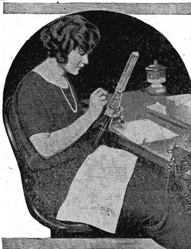
A girl's deft fingers formed the tongue with which S. S. Leviathan "speaks" at will by Radiotelegraph to either side the ocean. Miss Marie Frowick is seen assembling the "tongues" of a 10,000-watt vacuum tube. Two of these furnish the power to the Leviathan's big Radiotelegraph transmitter which has power enough to span the Atlantic. Western Electric Photo
