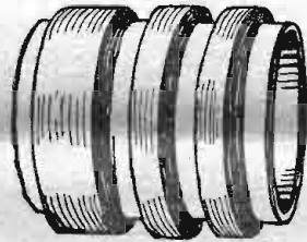
Figure 19—Bank-wound coil divided into sections
