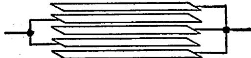
Figure 35—The first step in reducing the size of the two surfaces of a condenser for compactness
