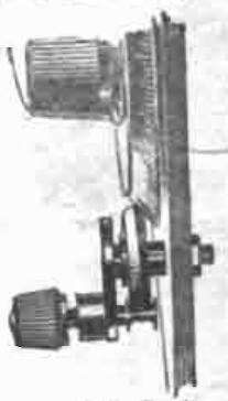
Pat. Pend. Side View showing friction drive against dial.
