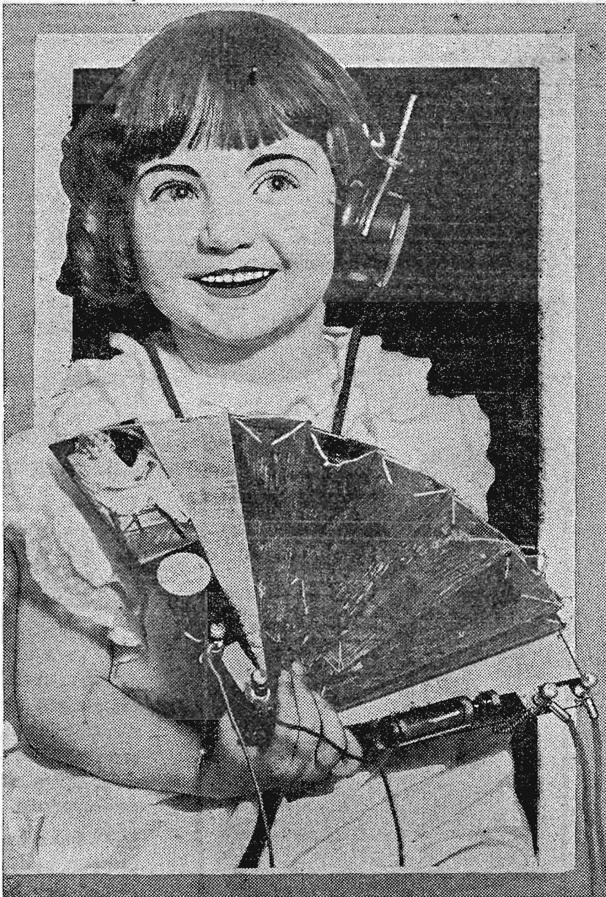
The first true Radio fan, literally speaking, is the one pictured above in the hands of Miss Mildred Nelson of Philadelphia, whose father has been nursing his hobby along by making some very odd types of receivers. The crystal detector and phone binding posts are on the right, and aerial and ground connections on the left. The inductance is tuned by opening or closing the fan. Mildred's dad also built her a book set, which was shown in the Digest recently. P. & A. Photo
