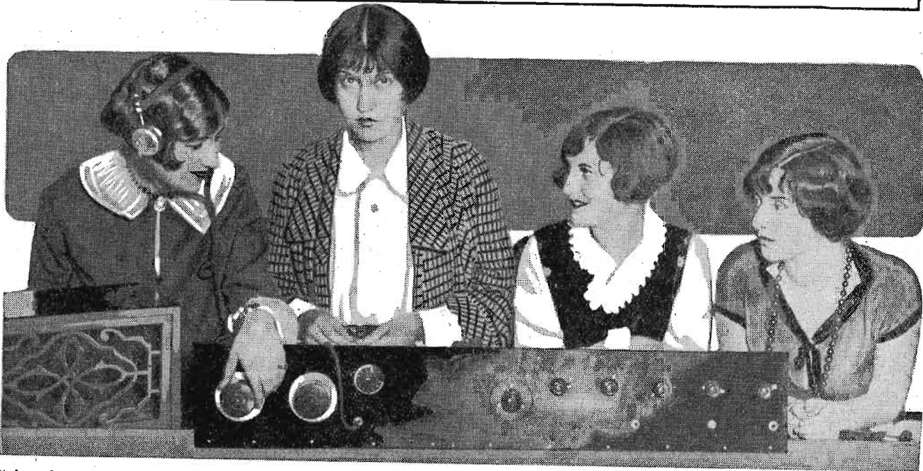
It is a far cry from the first one tube set in the experimental laboratories at Hunter College, New York, to the above photo. But, the girls have advanced to the super stage in the Radio division. They are shown assembling and testing a new eight tube super-heterodyne receiver with which they hope to "log" the coast regularly this winter.
