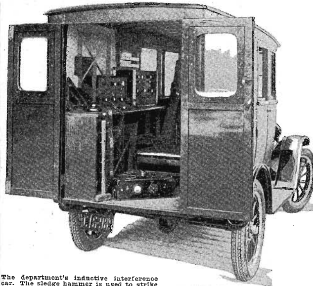
The department's inductive interference car. The sledge hammer is used to strike electric light poles in vicinity of the interference which will make and break a faulty circuit, and this is checked by another operator at the super-heterodyne on the bench.
