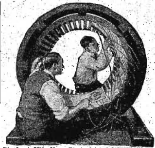
Student Winding Stator in COYNE Shops
