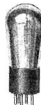
The amazing new RCA alternating current tubes—the UX 226 and UY 227—utilize for their filaments and their heating regular house-lighting current. Current is stepped down through transformers. Rectifiers are not used.
