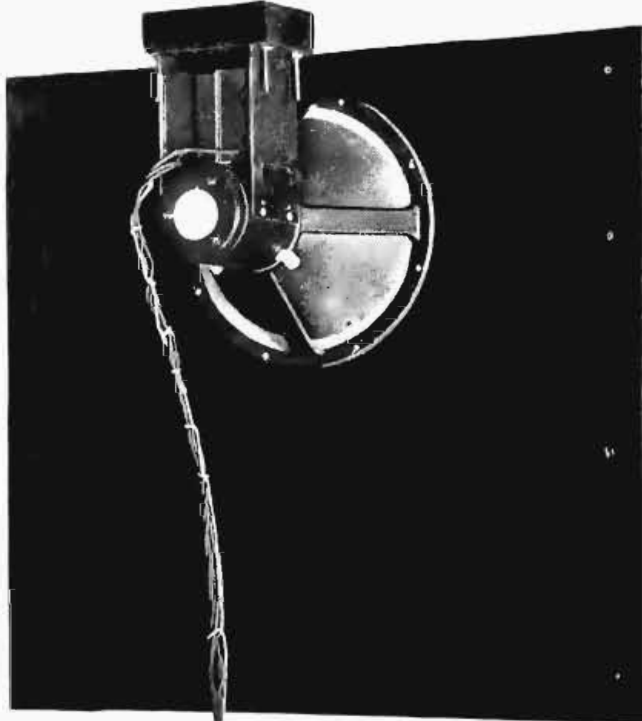
THE Jensen Dynamic Speaker is hung from ceiling of the lower compartment opposite the hole near top of baffle plate.
