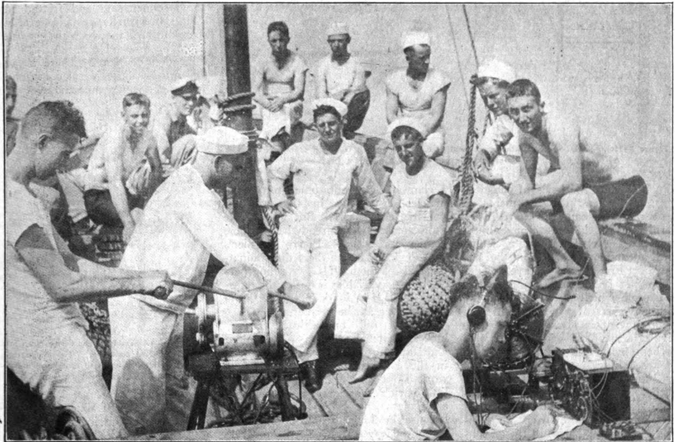
When a man goes down into the ocean's depths, today, he does not have to worry that the telephone cable will break. He gets his instructions and also talks to the ship above by radio. This photograph shows one of the pumps that supply the diver with fresh air and, alongside of it, the transmitting set that makes it possible to keep in touch with him by radio. The aerial for the diver is an insulated wire strung inside his air-cable. He uses a waterproof set strapped to his back. This set is tuned to the wave length of the ship afloat. While submarine wireless is quite an everyday affair, the communication between the diver and ship is a recent improvement.
