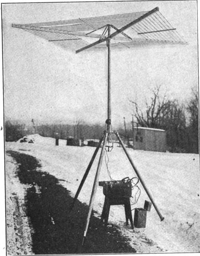
A fine photograph of a "loop," or "coil," antenna, or vertical conductor of electricity. The antenna is shown in place with a complete receiving-set. When supported by a six-stage amplifier, signals are received from France and Germany.
