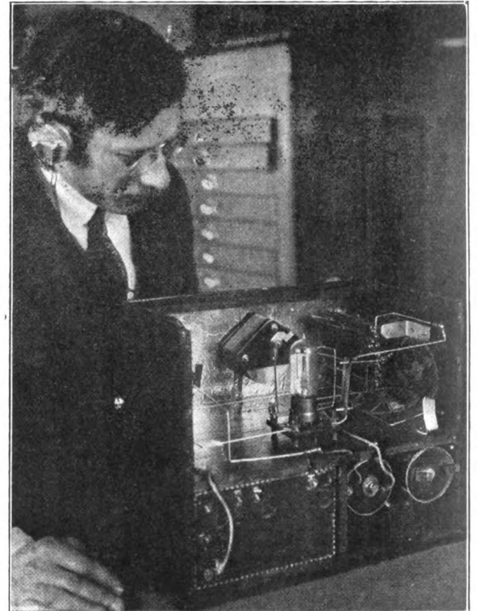
(C. Harris and Ewing) W. W. Tupper, of the Bureau of Lighthouses, and the receiving set he designed to make it possible for keepers of isolated lighthouses to keep in touch with the outside world. The set uses three spider web induc-tances to tune with and a WD-11 as a detector. As the Bureau has no appropriation to install the sets, blueprints and detailed instructions will be furnished by the Bureau to all keepers desiring them.
