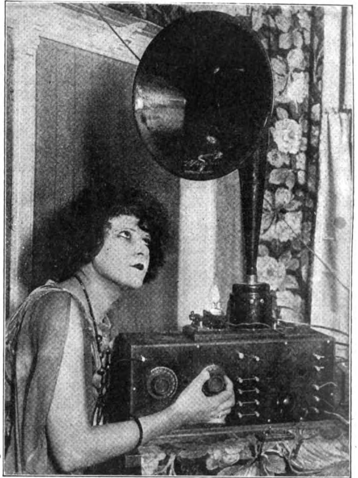
(C. Kadel and Herbert) A fair fan's idea that saves a lot of worry when she shuts off for the evening. Miss Margie O'Neil found that she sometimes went to her downy and forgot to turn the current off her Magnavox, with the result that the battery was run down the next morning. So she placed a small six volt lamp in parallel with the battery line, which warns her to "turn off."
