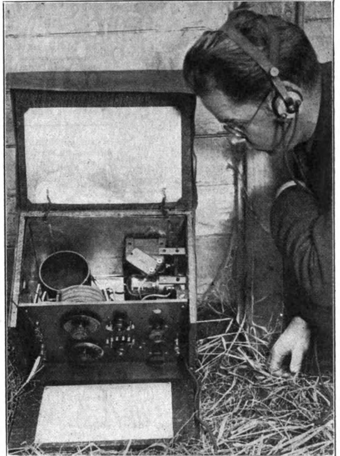
(C. Kadel & Herbert) (Above) The ideal set for the outdoor man. The set is absolutely water and weather proof. It was constructed by Wendell Kilmer to withstand any kind of weather. The set proper is regenerative, employing both radio- and audio-frequency. Excellent results have been accomplished using a barbed-wire fence as an aerial—and that in a pouring rain! As the photograph shows, the entire cabinet is shielded so that no capacity effect will be felt.
