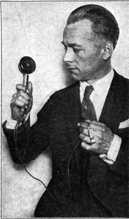
(C. Underwood and Underwood) Mr. Tracy T. Hicks, of Kansas City, Mo., and his new pocket wireless receiver, which is unique in that it is self-adjusting and no tuning or batteries are necessary. It is practically complete in itself. All that is necessary is to attach the clips to a suitable ground and aerial.
