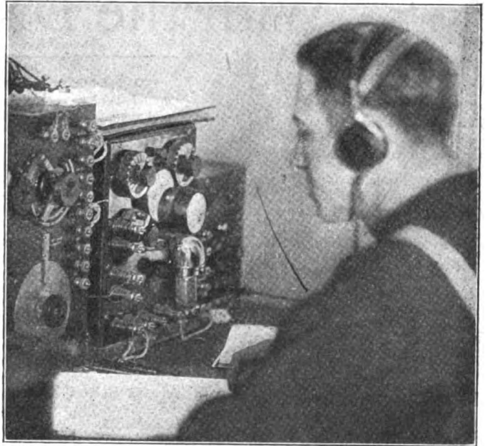
(Above) A corner of the radio room aboard a battleship. The photograph shows the long-wave receiver on the extreme right, and the separate tube-control cabinet. This apparatus is now obsolete, having been replaced with the more modern tube sets. However, it is used to train operators for warships. One of the most noticeable improvements that have been made in these sets is the fact that the tubes are now mounted on the inside of the cabinet. This guards against breakage. Another important fact: Instead of having connections on the front of the cabinet, these are all made at the rear. This makes a neater looking set. Because they are out of the way and cannot be fooled with, there is less chance of damaging the apparatus due to connections being loosened and, therefore, short circuited.
