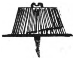
Figure 2—A completed knob made from a wooden spool.
