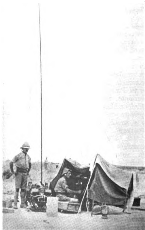
Pack Wireless Station.
