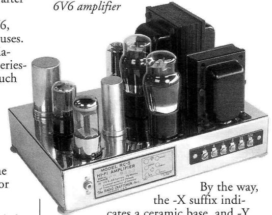
1948 RadioCraftsmen RC-2 10 watt 6V6 amplifier
