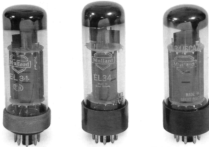
Mullard Type 1 Metal Collar Base, Type 1 Wide Brown Bakelite Base and Type 1 Dark Brown Bakelite Base
