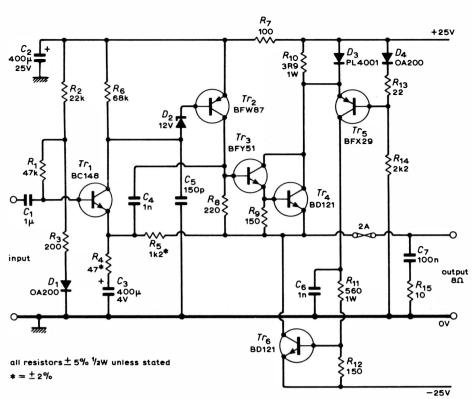
Fig. 3. Diagram of a 30W main amplifier utilizing the described technique.
