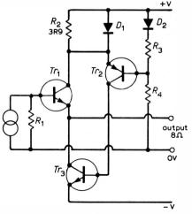
Fig. 2. Basic configuration of power output stage.
