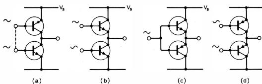
circuit quiescent current: at the point when the current in one transistor reaches zero the other has doubled. The peak load voltage remains at half the supply voltage when the output is biased to the supply mid-point for maximum undistorted output.
