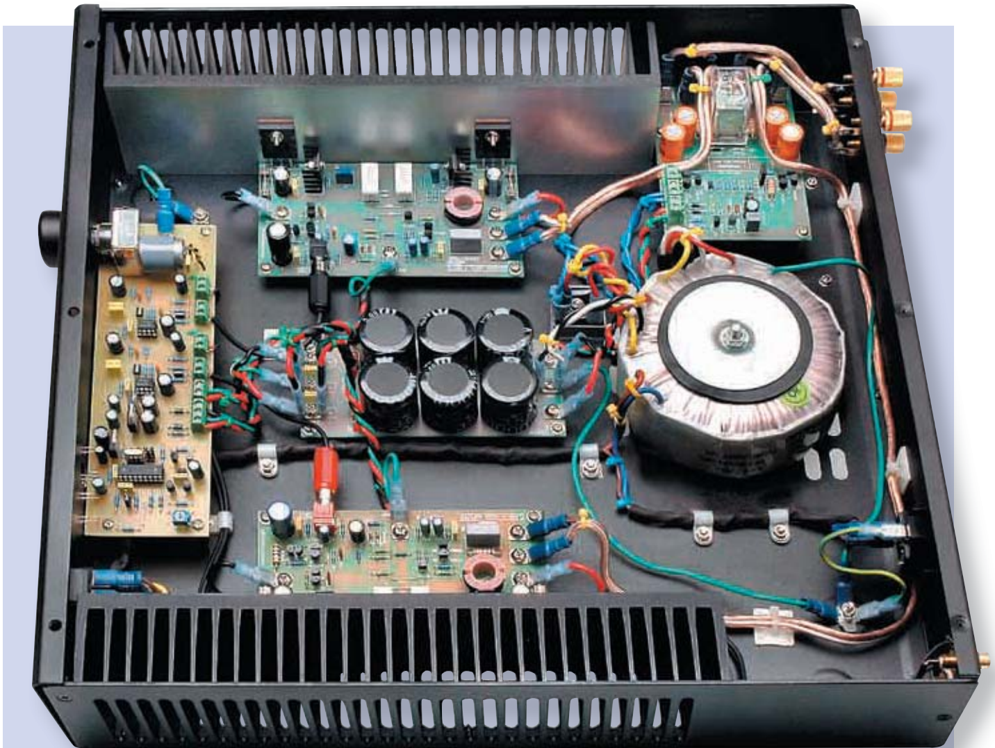
This chassis view clearly shows the routing of the loudspeaker cable from the right channel power amplifier. It runs along the bottom of the rear panel and is secured using adhesive cable tie mounts and cable ties.
