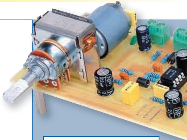
Fig.5: follow this parts layout diagram to build the Pre-amplifier & Remote Volume Control board. Be sure to use the correct part at each location and take care with components that are polarised. The leads to the motor are strapped to the underside of the board using cable ties.
