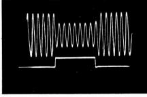
**Fig. 3.** Modulation of the reference voltage and the oscillator output voltage.
