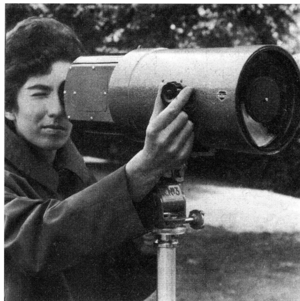
The image intensifier being demonstrated by Daphne Lampert, project leader of the group responsible for the early development of the tube.
