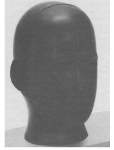
Neumann's artificial head shown mounted on its case.
