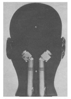
Showing the ear/microphone assembly of the Neumann "head".
