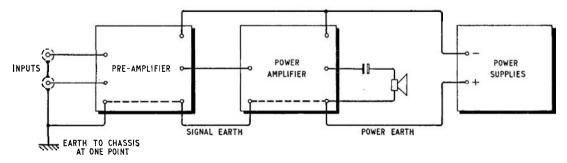
Fig. 9. Earthing diagram for power amplifier and associated equipment.
