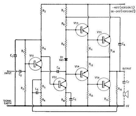
Fig. 4. Power amplifier circuit.
