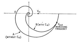
Fig. 8. Open-loop Nyquist diagrams of amplifier with (curve B) and without (curve A) the stabilizing capacitor  $C_A$ .
