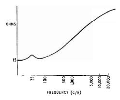
current gain falls appreciably at the high end of the audio-frequency band. However, this does not cause a corresponding reduction in performance because the impedance of a typical moving-coil speaker increases with frequency, see Fig. 7, (and hence the current it draws falls) at a rate which, in fact, more than offsets the decrease in current gain
