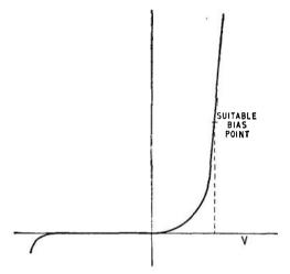
Fig. 5. Diode current/voltage characteristic.
