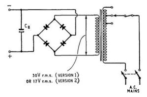
Fig. 6. Simple mains power supply circuit.
