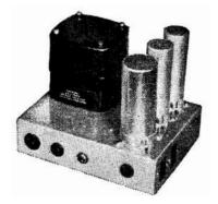
Power supply for stereo power amplifier and pre-amplifier.
