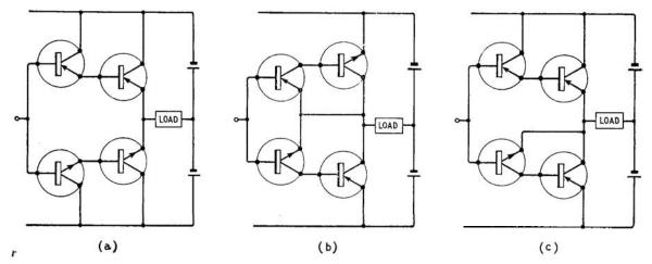
ig. 3 (a) Two-stage push-pull Class-B emitter follower. (b) Two-stage push-pull Class-B grounded-emitter amplifier with 100 per cent voltage feedback. (c) Hybrid circuit derived from (a) and (b).
