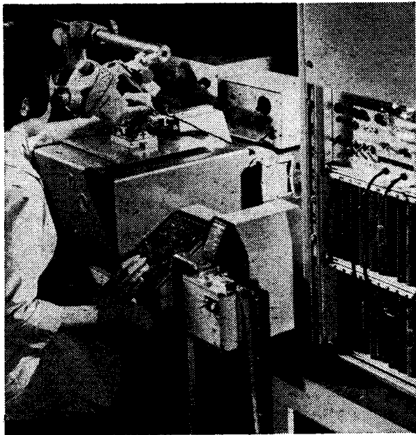
The illustration shows the equipment for micro-engraving of thin-film circuits. The control console for positioning of the table is shown on the right. In the centre is the tape reader and control box. The table with engraving head is on the left.
